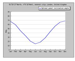
For example, the graph to the left was obtained showing how the optimum panel angle varies. The graph to the right shows the irradiation in London at an angle of 40°C. We can also get a figure of
